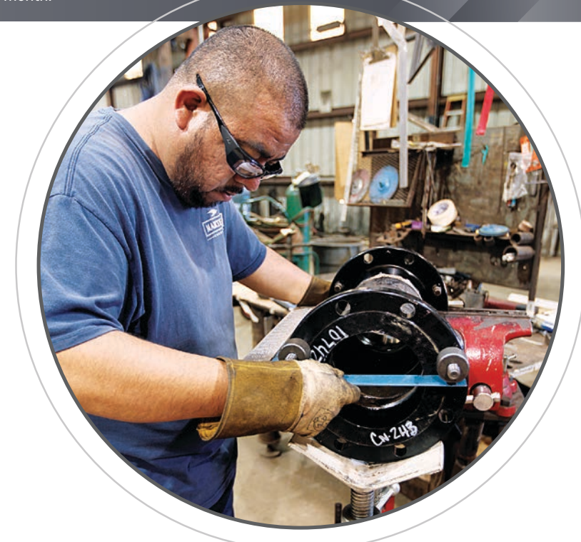
Fabricator Sergio Banda checks the fit on a flanged pipe spool.
